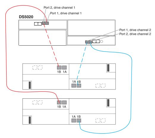
Figure 38. Cabling for one DS5020 and two storage expansion enclosures
